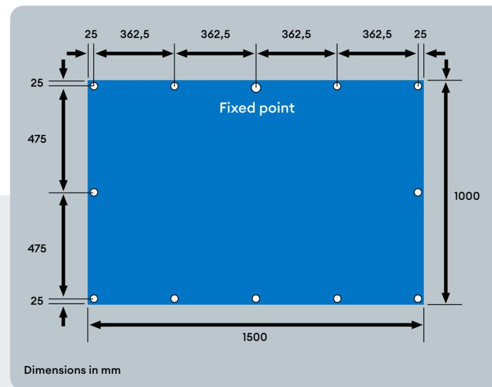
Furthermore, the hole centre distance from the edge of the sheet should be at least 2.5 times larger than the drilled hole.
