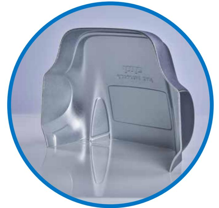
sheets are prestretched pneumatically, i.e. by air. These processes are the ones that generally produce thermoformed parts with the most uniform material thickness.
